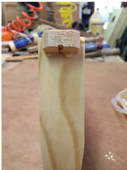
Figure 8 – A properly glued top and end bar. You know that you have added enough glue when glue bleeds from the joints once the parts are assembled.
