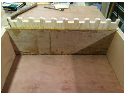
Figure 20 – Using a jig to facilitate frame assembly. In this jig, 10 end bars are inserted into a special compartment made to accommodate them.
