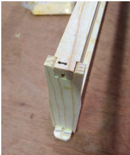
Figure 12 – A staple properly driven through the bottom bar and into the end bar.
