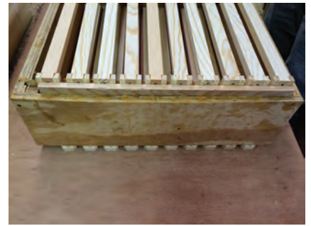
Figure 26 – In this jig, a wooden wedge that runs the width of the jig is inserted between the frame end bars and the wall of the jig. Similarly, a wedge is added to the other side. These wedges square the frames prior to driving the fasteners through the bottom bar and into the end bars.
