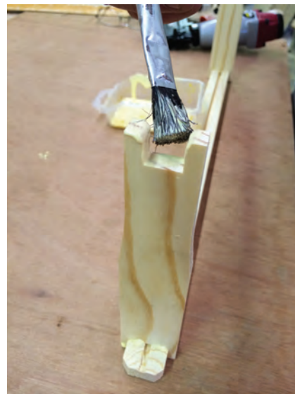
Figure 10 – Applying wood glue to the notch at the bottom of an end bar.
