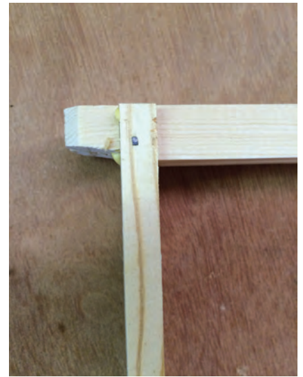
Figure 17 – A nail driven through the side of the end bar and into the top bar. This nail complements the staples driven (1) from the top of the top bar and into the end bar and (2) the face of the end bar and into the rib of the top bar. Thus, there are fasteners driven into the top/end bar joint in three directions, the X, Y, and Z axes.
