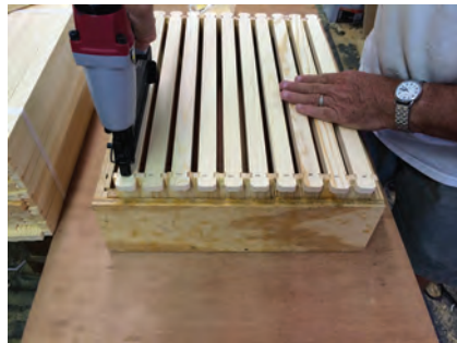
Figure 23 – Using a staple gun to drive staples through the top bars of frames and into the end bars.
