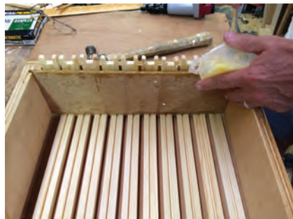
Figure 24 – The jig is flipped and glue applied to the bottom notch in the end bars.
