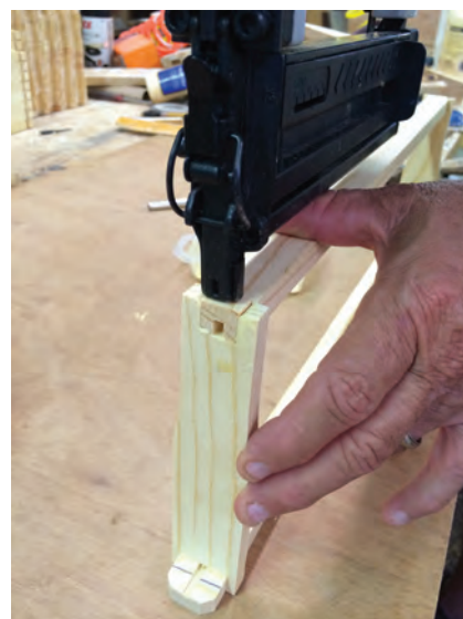
Figure 11 – Driving a staple through the bottom bar into the end bar. Notice how the staple is being driven to the left of the groove in the bottom bar. This ensures that the staple is driven exclusively through solid wood.
