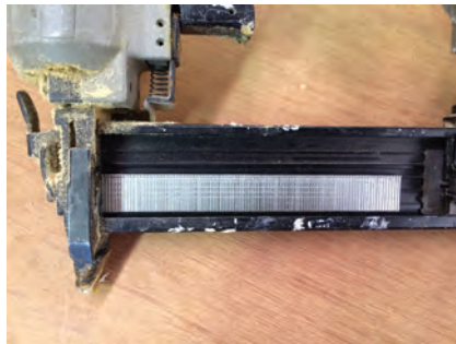
Figure 16 – This nail gun drives small nails, the type that is good to drive through the top and bottom sides of the end bars and into the top and bottom bars, respectively. 3/4 inch nails can be used for this purpose.
