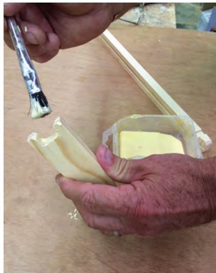
Figure 7 – Applying wood glue to the upper notch in an end bar using a paint brush.
