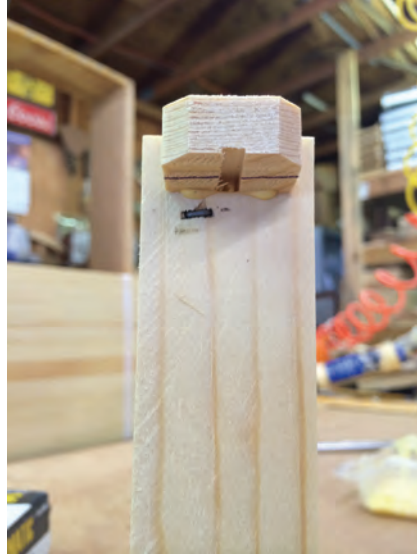
Figure 14 – The staple driven through the face of an end bar and into the rib of the top bar.
