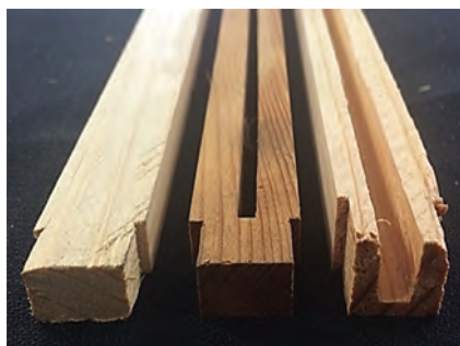
Figure 4 – Three styles of frame bottom bars. They include solid (left), split (middle), and grooved (right).
