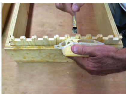
Figure 21 – Wood glue being applied to the upper notches in the end bars.
