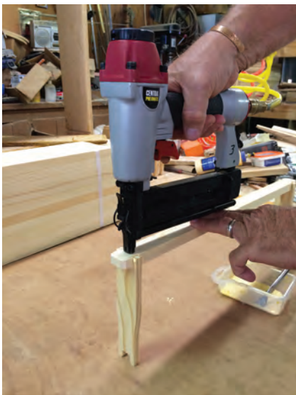
Figure 9 – Using a staple gun to drive a staple through the top bar of a frame and into the end bar of a frame. The staple gun is powered by an air compressor.
