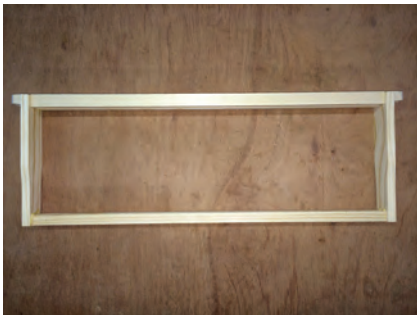
Figure 15 – A frame resting on a flat surface and waiting to receive the nails that are driven through the sides of the end bars.
