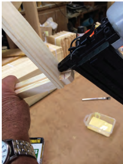
Figure 13 – A staple is being driven through the face of an end bar and into the rib of the top bar. This, in my opinion, is the most important fastener added to a frame. This single fastener will keep the top bar of a frame from being pried from the end bars in normal circumstances.
