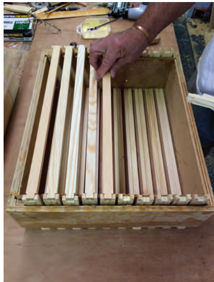
Figure 25 – The bottom bars are added to the end bars.
