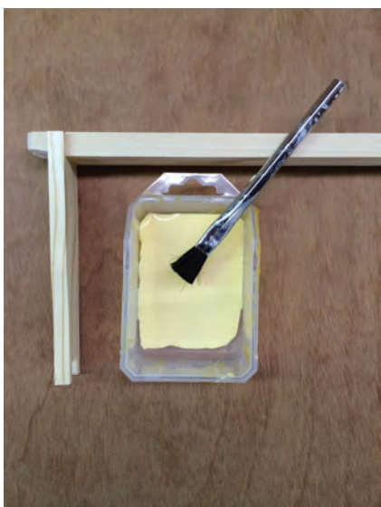
Figure 5 – Wood glue can be put into a plastic container to make it easier to apply to the frame parts. A brush can be used to apply the wood glue to the various frame parts.
