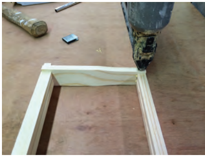
Figure 18 – A nail being driven through the bottom side of the end bar and into the bottom bar. This single nail keeps bottom bars from pulling away from the end bar under normal frame use.
